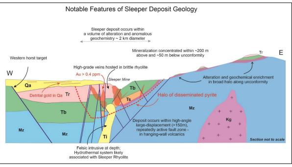
Figure 6-5: Schematic Cross-Section Model of the Sleeper Deposit
